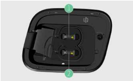
1. AC slow charging port 2. DC fast charging port
